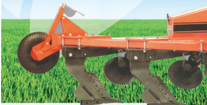
PARA PLOUGH is now available for sub surface aeration. This is the ultimate machine to fracture under the surface while still leaving a level surface. The angled leg is what makes the difference!
